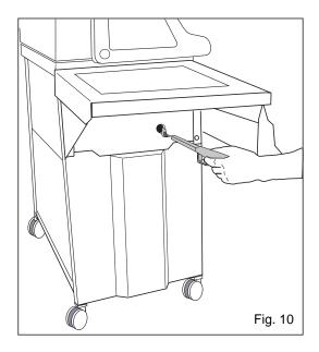
5. Turn the <u>left</u> Burner Control Knob to the HI position by pushing down on the knob and turning it counterclockwise.
